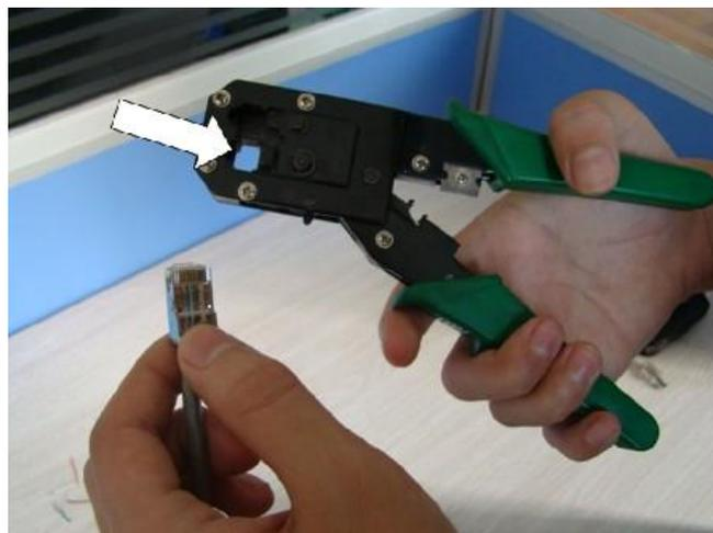
See the following photo for the pressed plastic joint and unpressed plastic joint. The left one is pressed, whose copper pressing knife is fully sunk in the plastic joint, as shown below.
