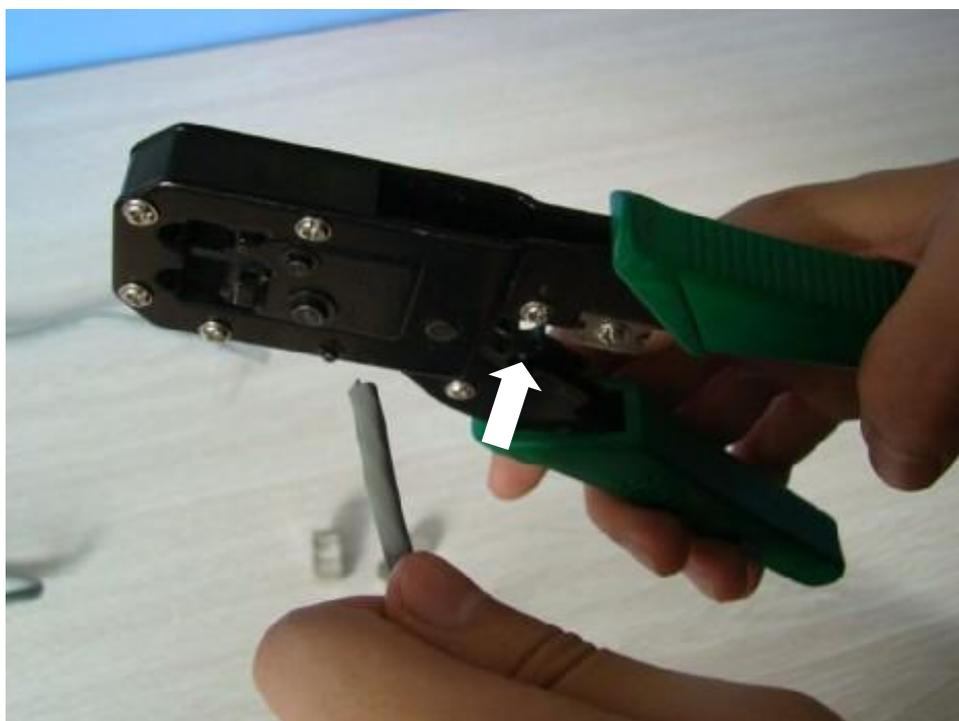
**Step 2:** Stripe 1.5cm external protective shell at one end of twisted pair with the wire stripper of RJ-45 crimping pliers (the joint will be loose if the stripped shell is too long and its metal knife edge cannot fully touch with core wire if the stripped shell is too short). The core wire shall not be damaged, as shown below:
