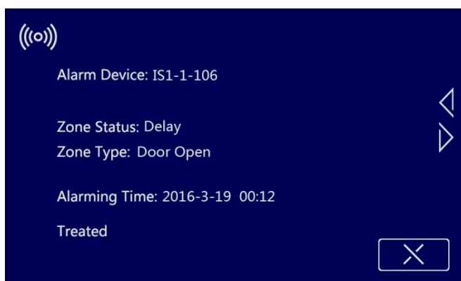
Figure 2.7 Door opening alarm interface
