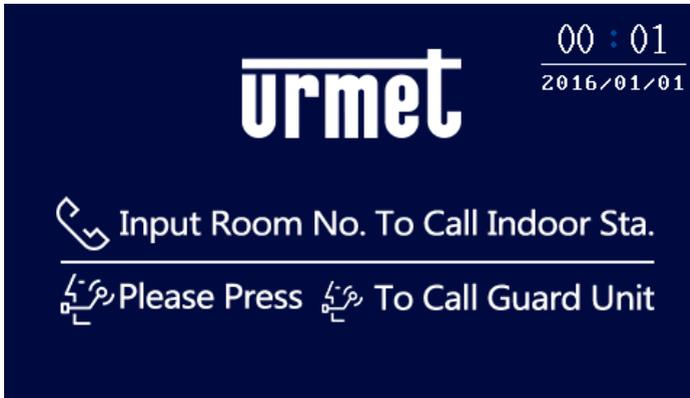
At standby interface, press "#" key and then press " \* " key to enter into engineering setting login interface. **The default engineering setting password is "000000".**
